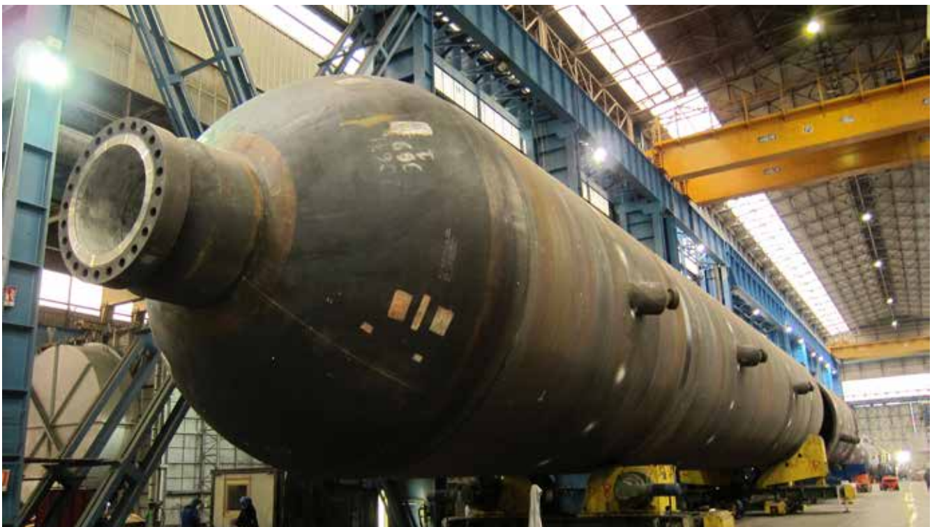
The reactors, based on Mild Hydrocracking technology and UOP process, will be among the largest ever built worldwide.
