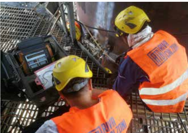
TODFT Ultrasonic test on Mangalore reactors
